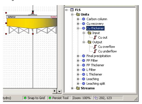
New <u>Stream and Unit Navigator</u>: using the navigator will give you better control over how streams are connected. Selecting a unit or a stream in the navigator will also show the selection in the flowsheet and vice versa. If a unit or stream is on a different page, HSC Sim will select and show that page. The navigator has a "Highlight Streams" feature: applying it will highlight the input (colored blue) and output streams (colored red) of the selected unit.
