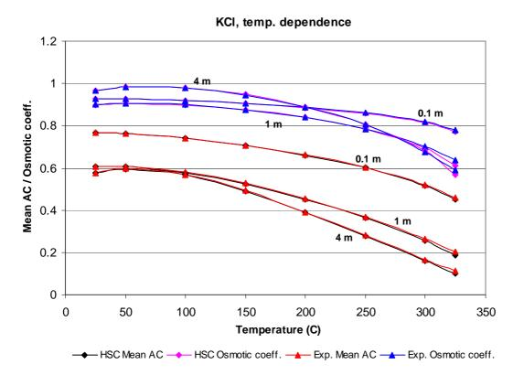
The enthalpy aqueous solutions and especially the activity coefficients depend on the concentrations of the species. The new Aqueous Estimator module provides you with an easy way to estimate activity coefficients, enthalpies and heat capacities of dilute, moderate, and concentrated electrolyte solutions as a first guess for process design purposes.
