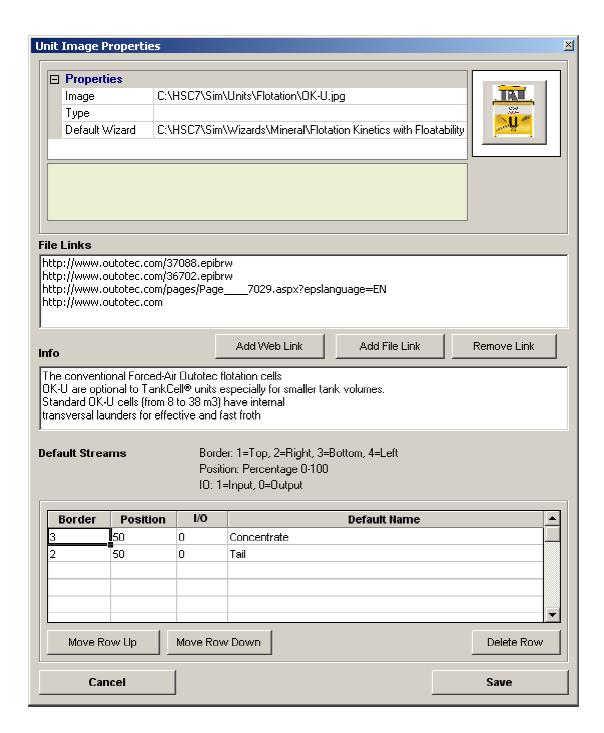
The unit icons may be connected with Model Wizards (Particle and Reaction mode), unit models (Distribution mode), Internet and file links. These file links may be used to give more information of the process units. These file links are also available in the flowsheet behind the unit icons.
