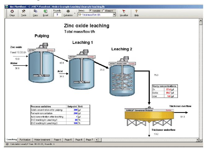
HSC 7 has multiple <u>new high-resolution icons</u> for different unit processes. The unit icons are grouped under the following folders: Acid Plan, Analyzers, Experimental, Ferro, Flotation, General, Grinding, H2SO4, Hydro, Iron&Steel, Minerals-Others, Others, Physical Separation, Precious Metals, Pyro, Roasting, Thickeners.
