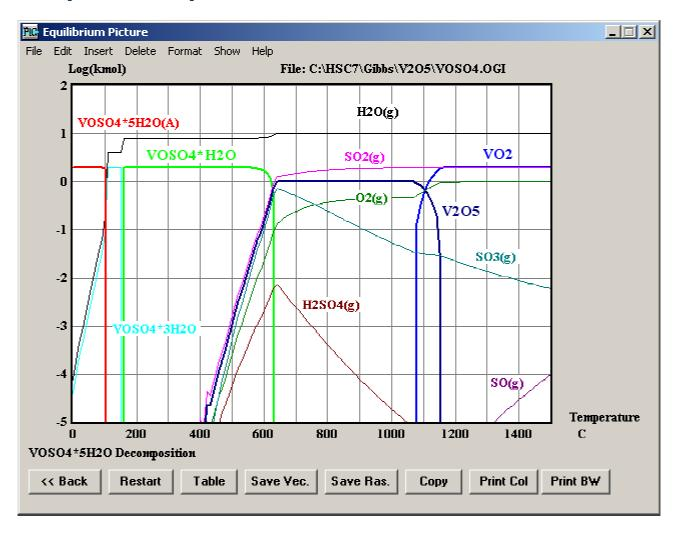
The HSC Equilibrium module calculates unit process output at the equilibrium state when the user specifies the chemical system and the raw materials. This module uses the Gibbs Energy Minimization method, which takes all the possible chemical reactions into account automatically.
