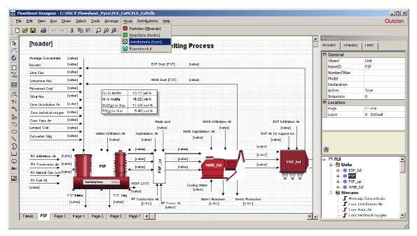
The Sim flowsheet module was originally made for the simulations of chemical reactions and mineral processing. The new Distribution (Pyro) mode also makes it more feasible for high temperature process models, which are based on the distributions of elements.
