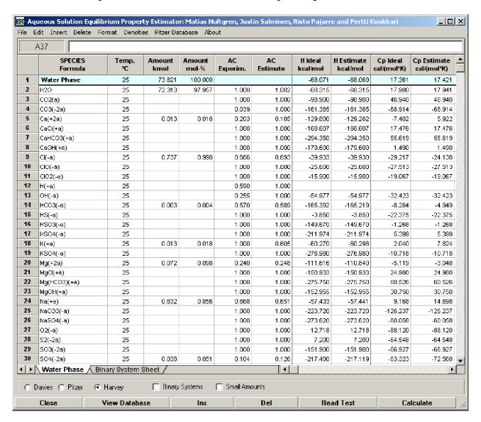
Aqueous solutions are widely used in the process industry in a huge number of applications. Process models may be created using pure substance data and assuming ideal behavior for the aqueous solutions. However, the accuracy of the models may be improved by taking into account the naturally existing non-ideal behavior of ions in the solution.
