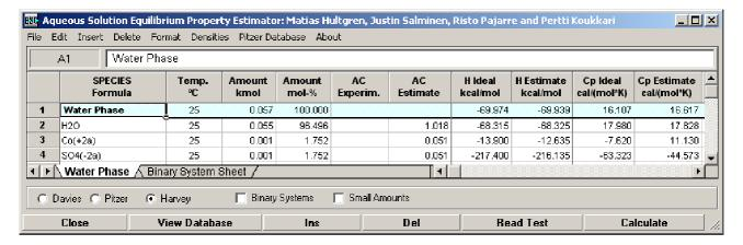
The HSC Aqua **Binary System Sheet** can be used for calculation of activity coefficients, osmotic coefficients, enthalpies of solution, and heat capacities of binary electrolyte systems. These include for example NaOH, KOH, NaCl, KCl, HCl, LiCl, CaCl<sub>2</sub>, ZnCl<sub>2</sub>, Na<sub>2</sub>SO<sub>2</sub>, CaSO<sub>4</sub> CuSO<sub>4</sub>, CoSO<sub>4</sub>, NiSO<sub>4</sub>, MgSO<sub>4</sub>, MnSO<sub>4</sub>, ZnSO<sub>4</sub>, AgNO<sub>3</sub>, and many others.
