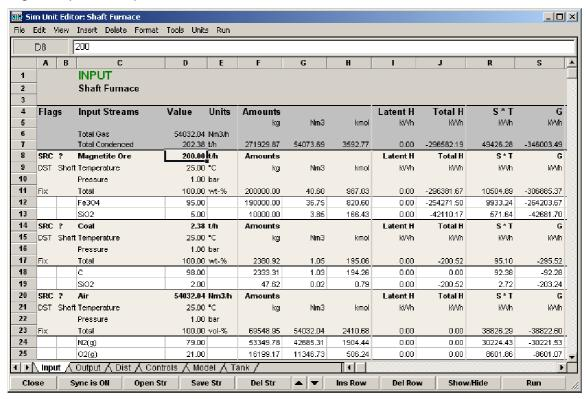
The distribution mode handles streams as rows unlike the Reaction and Particle modes, where each stream reserves one column. These streams may be saved to the stream database and reused in some other process model. The lack of a fixed variable list makes Distribution mode streams and units easier to reuse in the other process models. The Distribution mode behaves more like the old HSC Balance module.
